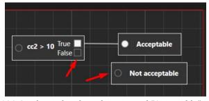
Figure 7.130 Conditional node with connected "Acceptable" result node
