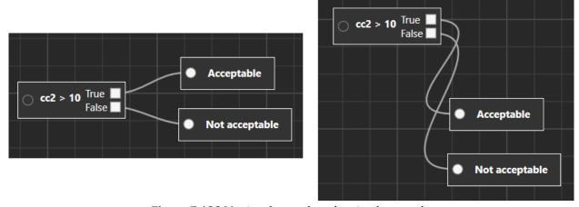
Figure 7.138 Moving the result nodes simultaneously
